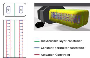
Figure 4: Constraints set up in Simulation as fixed distance constraints
