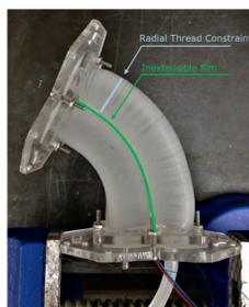
Figure 2: Single link with constraints highlighted
