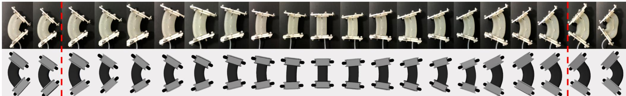
Figure 5: Visual comparison of link expansion after settling from -10 to 10 psi pressure. Negative values mean the left chamber is inflated, while positive values are for the right chamber. The simulation displays high accuracy on the curvature up to 8 psi, where the dashed lines were traced. After that the pressure becomes excessive and the real link stops following the linear model
