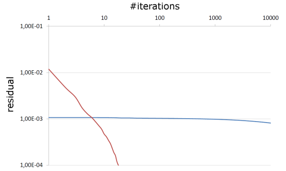
Fig. 6. Typical convergence behavior for a GMRES solver using our preconditioner (red line) and without a preconditioner (blue line) in a flow dominated by surface tension. In this example, preconditioning helps GMRES converge to a desired final residual of 10^{-4} in as few as 20 iterations.
