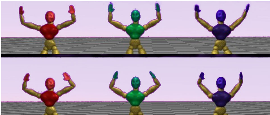
Fig. 6 Comparison study of animation quality when using box-limits versus signed distance-fields. The figure on the left shows signed distance-fields, the figure on the right shows box-limits. The figure in the center is the motion capture reference
