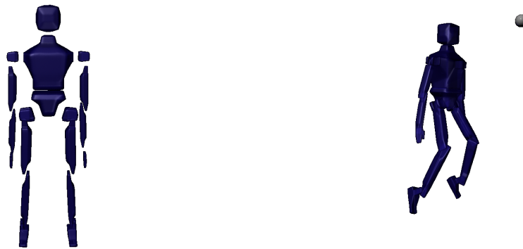
Figure 2: A robot assembles itself during simulation using constraint stabilization. Simulation was done using a velocity based complementarity formulation. Complementarity problems were solved with Path [115]. Rendering was done using Maya ® .
