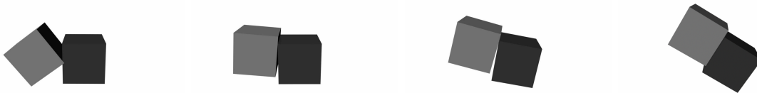
Figure 4.31: A sequence in a first order world simulation where two objects of different mass are aligned. The left box has less mass than the right box. The left box is pulled to the right. Observe that the heavier box on the right is less affected than the light box on the left in comparison with Figure 4.30.
