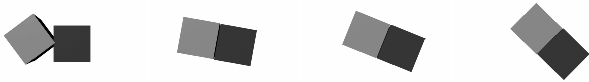
Figure 4.30: A sequence in a first order world simulation where two identical objects are aligned. The left box is pulled to the right. Observe that both the left and right boxes are equally affected.
